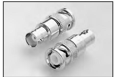
**Model 7078-TRX-GND:** 3-slot male triax to female BNC adapter (guard removed) for adapting non-guarded measurements to the Model 7072 or 7072-HV Semiconductor Matrix Cards or 8006 or 8008 Test Fixtures.
